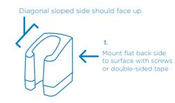
Place camera bottom (the side where the USB connector sits) through the cradle top-opening.
